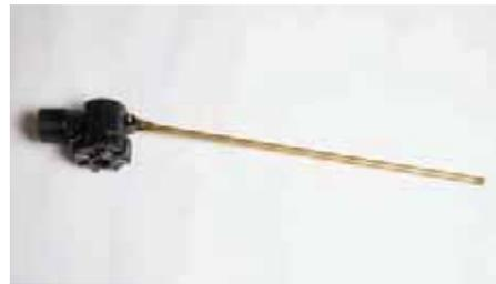
A diffuser is built into the outlet to break up the water jet and reduce trough turbulence. While the float arm is thin, it is a tensile brass alloy and does not bend easily.
