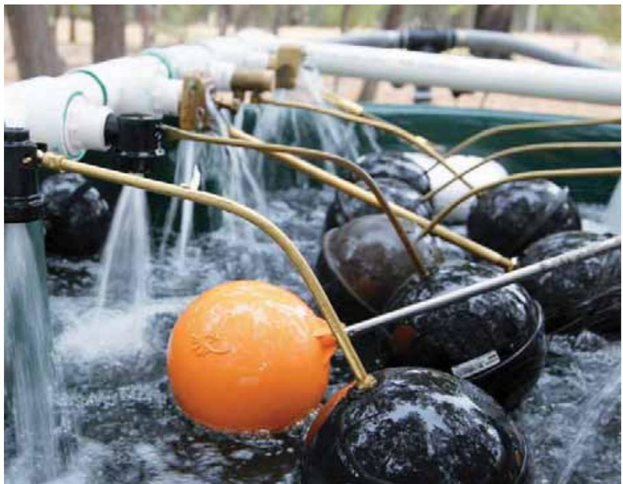
*Kondinin Group engineers mounted 15 valves in one trough and cycled them 20,000 times to simulate an average working life. Apart from normal wear and tear, no valves actually failed during testing, leading engineers to conclude the vast majority of valve issues are caused by incorrect application, stock damage or poor water quality.*
