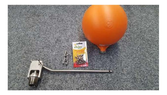
With the trough inlet being vertical at the bottom we designed a unique arm that allows our valve to be mounted vertically and the valve arm sit just 35mm above the bottom of the trough when fully open and then moving up away from the bottom of the trough as the valve shuts off. When the valve is fully closed the end of the arm is only 150mm above the bottom of the trough.
