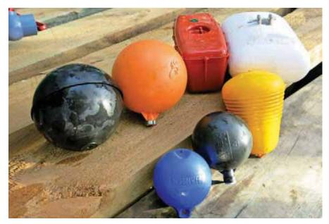
Floats are a pretty important, but often overlooked, part of the system. Make sure the threads are in good condition, and any locknuts on the float arm are tightened against the valve. Floats pictured (clockwise from left) are the Philmac 150mm, Cocky valve, Philmac Stockproof, Raindrop, Jobe, Hansen Max-flo and Apex Xtraflo.
